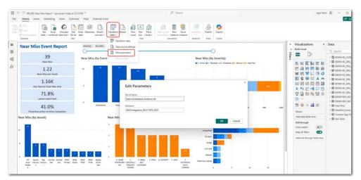
For BI Reports published to customers, the parameters can be accessed in Power BI Workspaces under the **Parameters** setting, where the Server Name and Database Name will be updated based on the standardised parameters using the customer's Server and Database Names.
